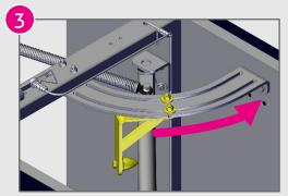
Open the return door completely. Move the handle and tighten the nut locks to fix the door.
