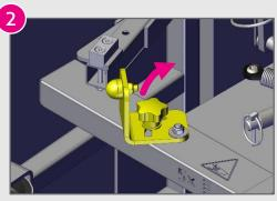
Open the doors of the *entrance gate* completely. Move the gate openers by turning the knob and fix them.
